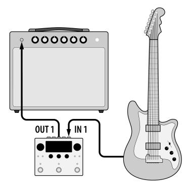
Fig. 3.2 A simple mono guitar configuration
