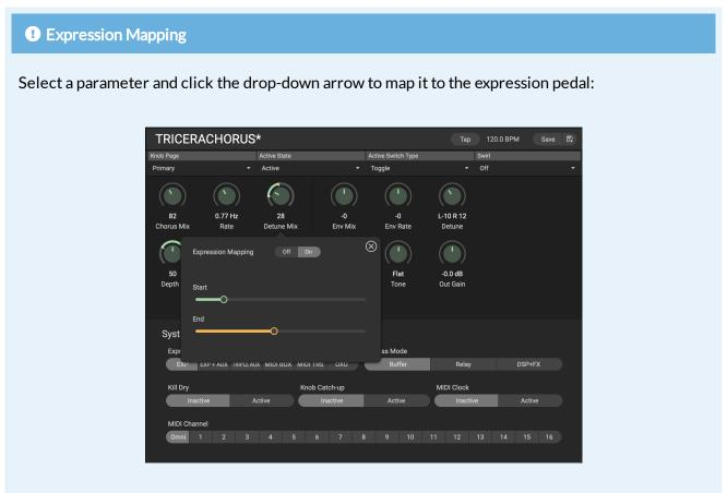
Fig. 10.20 The Detune parameter is mapped to the expression pedal.
