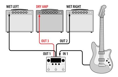
Fig. 3.9 Wet/Dry/Wet guitar amp configuration
