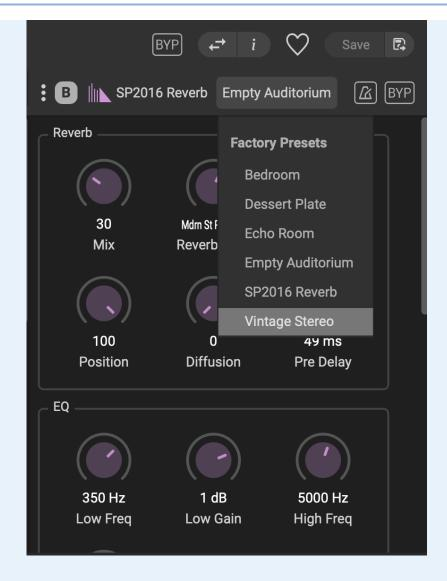
Fig. 10.7 SP2016 Reverb's preset dropdown menu for Preset B.
