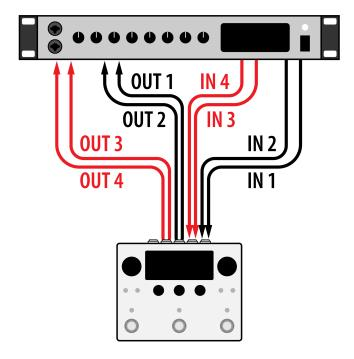
Fig. 3.12 Dual Inserts are connected to an audio interface
