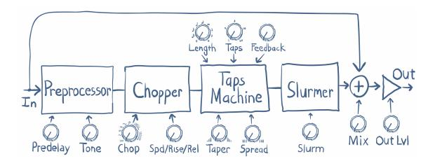
Fig. 2 UltraTap's signal flow diagram
