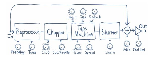
Fig. 2 UltraTap's signal flow diagram
