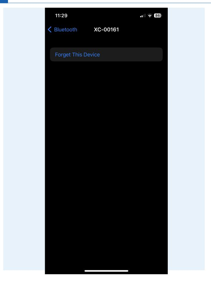
Fig. 7.33 Forget the H90 on your iOS device before pairing again.
