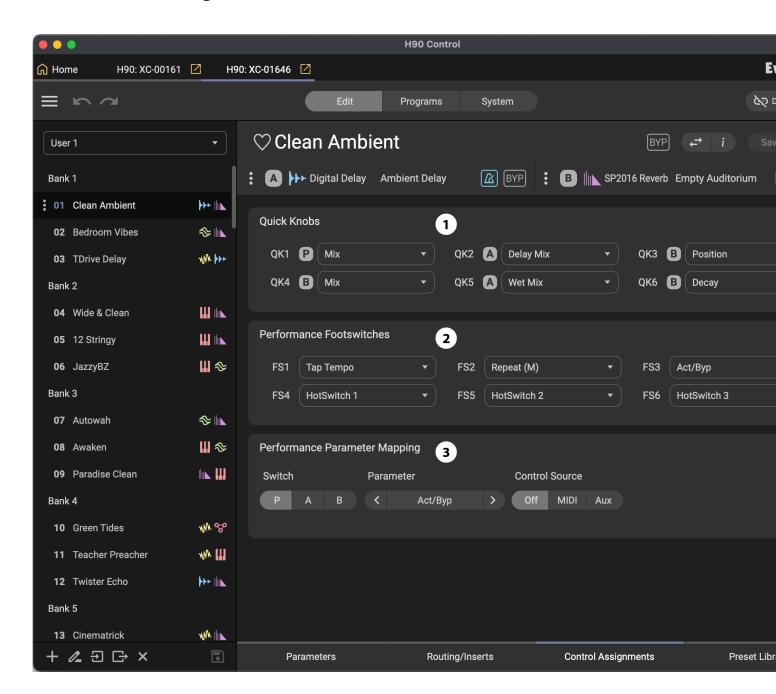
Fig. 10.8 The Controls Assignments edit menu.
