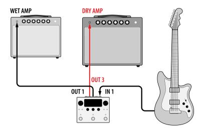
Fig. 3.6 Wet/Dry guitar amp configuration
