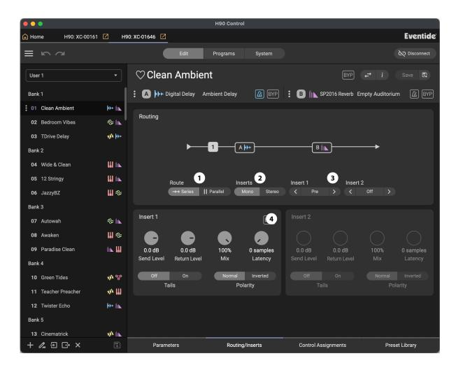
Fig. 10.8 The Routing/Inserts edit menu. Insert 1 is Pre Preset A.
