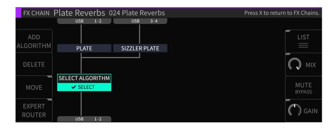
In the H9000, each FX chain can contain up to four separate signal processing algorithms. The *Algorithms* screen is where you work with these algorithms; you can navigate to it by:
