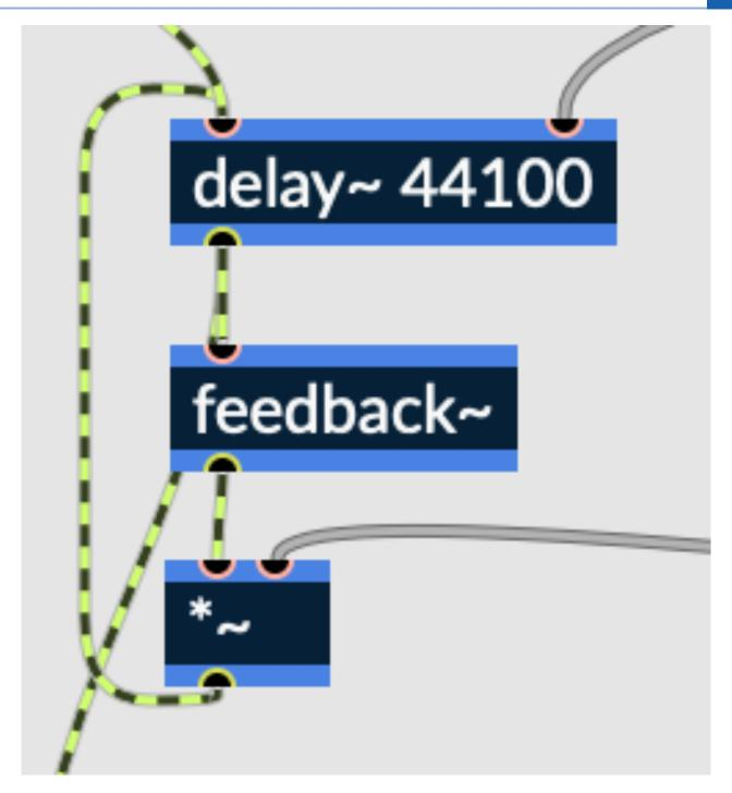
Fig. 6.96 Delay feedback loop
