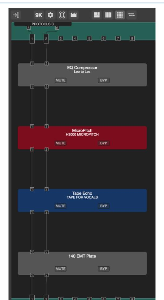
Note that the H9000 displays the expansion card I/O as a single 32-channel device, while Pro Tools divides the I/O into two separate 16-channel devices. In the above example, expansion card I/O 1-16 will appear in Pro Tools as **C 1-16**, while expansion card I/O 17-32 will appear in Pro Tools as **D 1-16**. For example, if you want to route your audio into HD expansion inputs 19-20, they will appear in Pro Tools as **D 3-4**.
