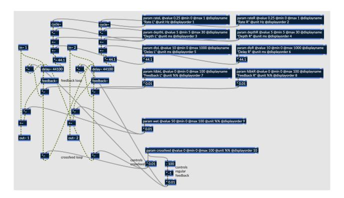
Fig. 6.105 Stereo flanger patch with crossfeed in RNBO
