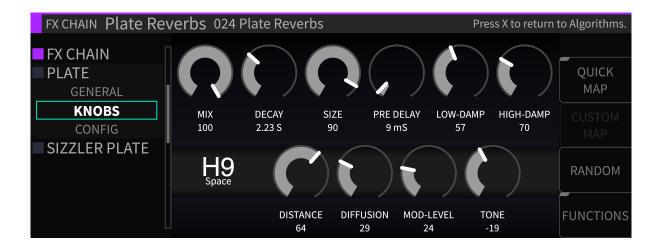
Each algorithm contains a set of parameters; you adjust these parameters to adjust the sound of the algorithm you have selected.
