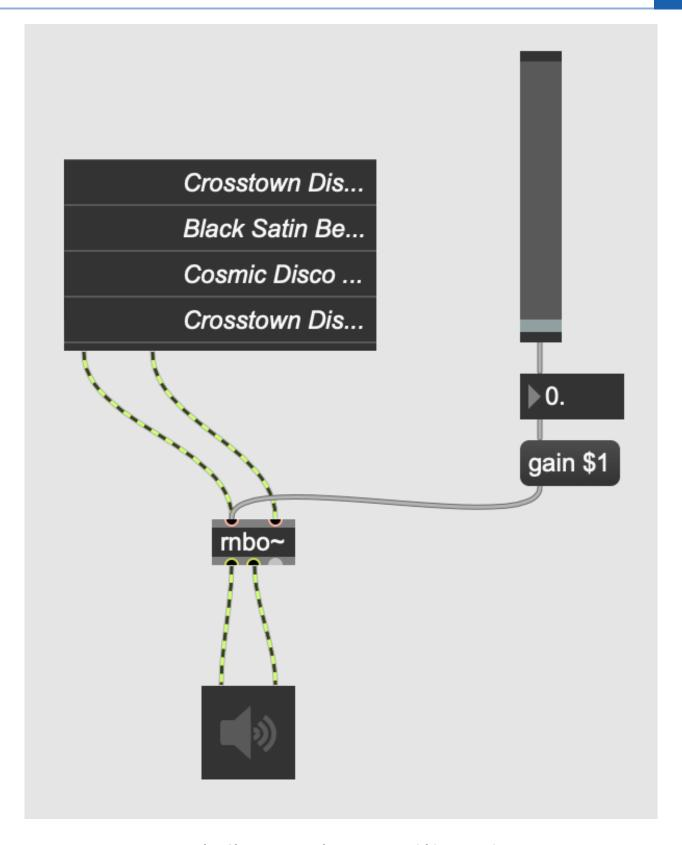
Fig. 6.77 Example of how to control parameters within Max using messages
