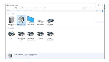
The H9000 will now appear as an audio device in the Windows "Devices and Printers" control panel, and its audio inputs and outputs can be used with any ASIO compatible software.
