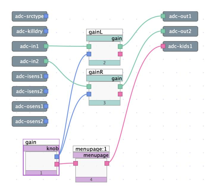
Fig. 6.13 Simple gain algorithm, with the addition of a knob and menupage to allow for user control
