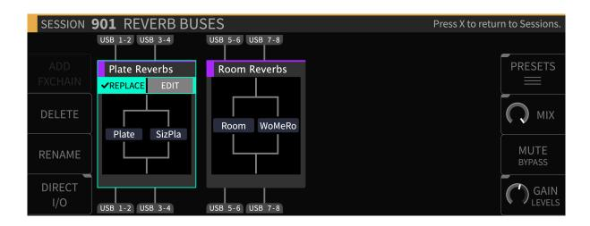
Press the front panel FX Chains button to switch the display to the FX Chains view screen, where you can view and edit the FX chains of the currently loaded session.
