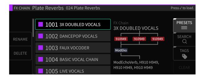
At any time, you can press the *Cancel* button to back out of the current screen state and return to the previous state. Pressing the *Cancel* button a final time will exit the *FX Chains* screen and return you to the *Sessions* screen. You can always return to the *Sessions* screen by pressing the *Cancel* button once for each iteration of menus you have entered. In other words, if you're in too deep and need to reset, press the *Cancel* button to get back home.
