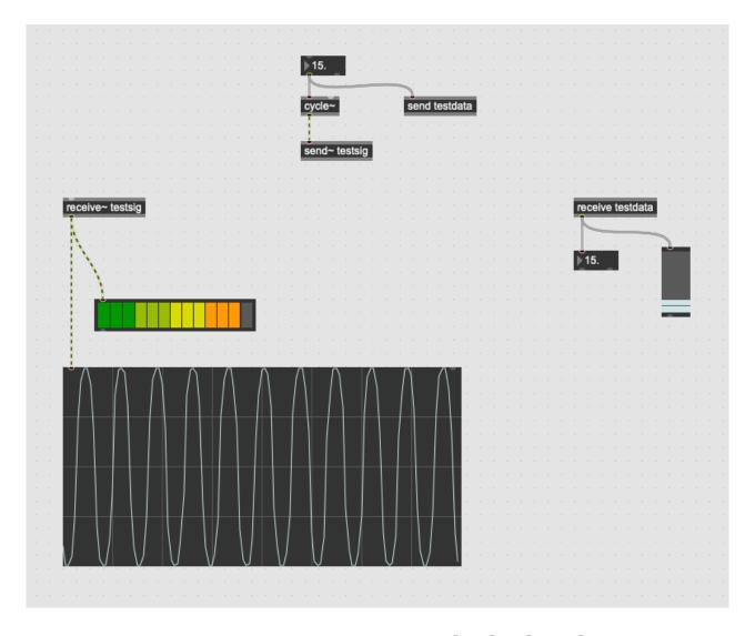
Fig. 6.61 Basic Max patch demonstrating [send] and [receive]
