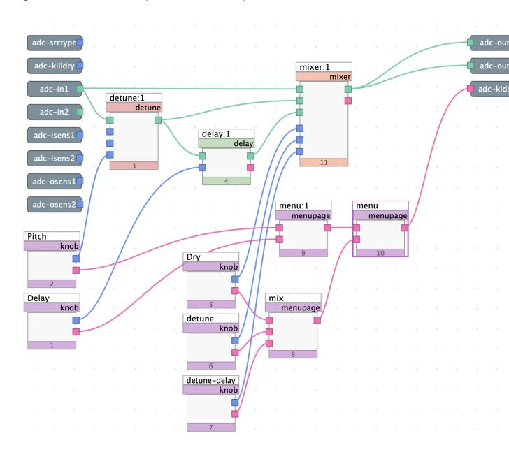
Fig. 6.25 Simple chorus effect with several interface modules and menupages
