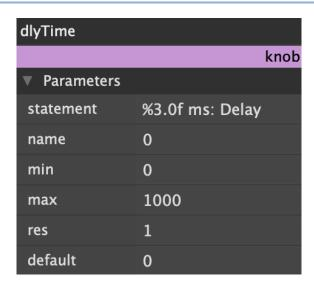
Fig. 6.8 Knob module utilizing %f syntax in its statement field
