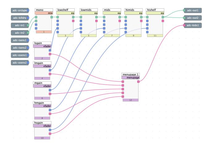
Fig. 6.27 5-band graphic equalizer algorithm
