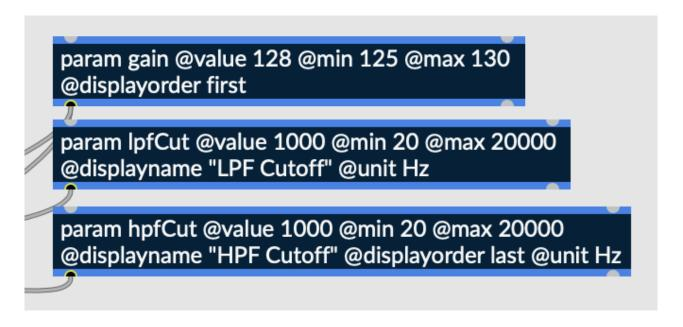
Fig. 6.81 Param objects, controlling gain, LPF cutoff frequency, and HPF cutof frequency
