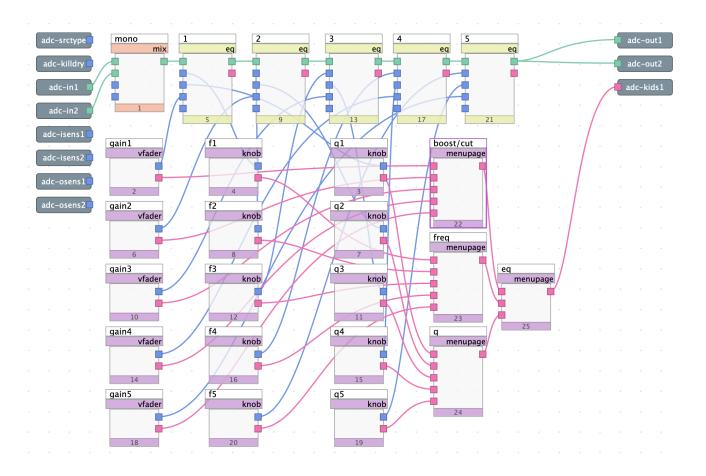
Fig. 6.29 5-band parametric equalizer algorithm
