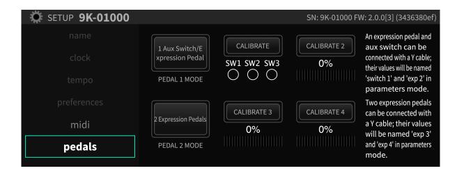
The H9000 allows connection of up to four independent foot pedals; these pedals can be a "switch" type (on/off) or a "continuous" type (volume) pedal.
