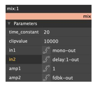
Fig. 6.4 Editor page for a mix module. All parameters are shown, including signal inputs and their associated amplitudes.
