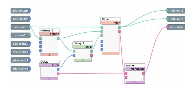
Fig. 6.22 Simple chorus algorithm with one knob
