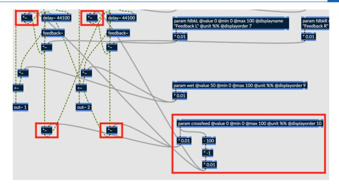
Fig. 6.108 Crossfeed param controls four \*~ objects simultaneously, maintaining a balance between feedback and crossed feedback
