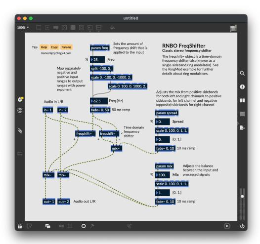
Fig. 6.52 The RNBO FreqShifter patch.
