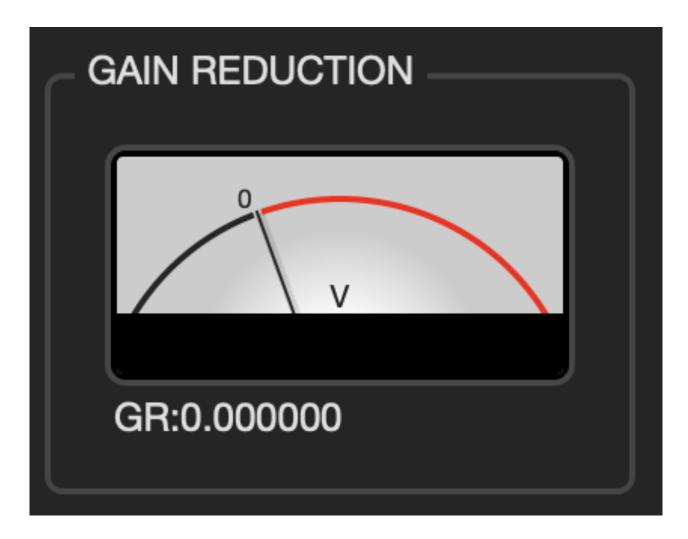
Fig. 6.42 Analog style meter used to show gain reduction
