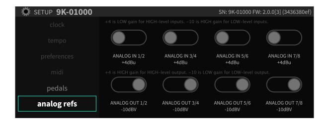
The Analog Reference Levels screen allows you to set the levels for the eight analog inputs and outputs present on the DB-25 connectors. This allows the H9000 to be installed in a wide variety of environments, and interface at an optimum level with professional and some consumer equipment.
