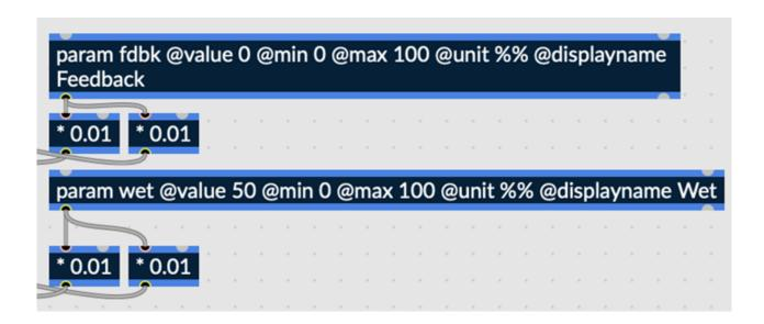
Fig. 6.98 Feedback and wet control param objects, both scaled by 0.01 on output
