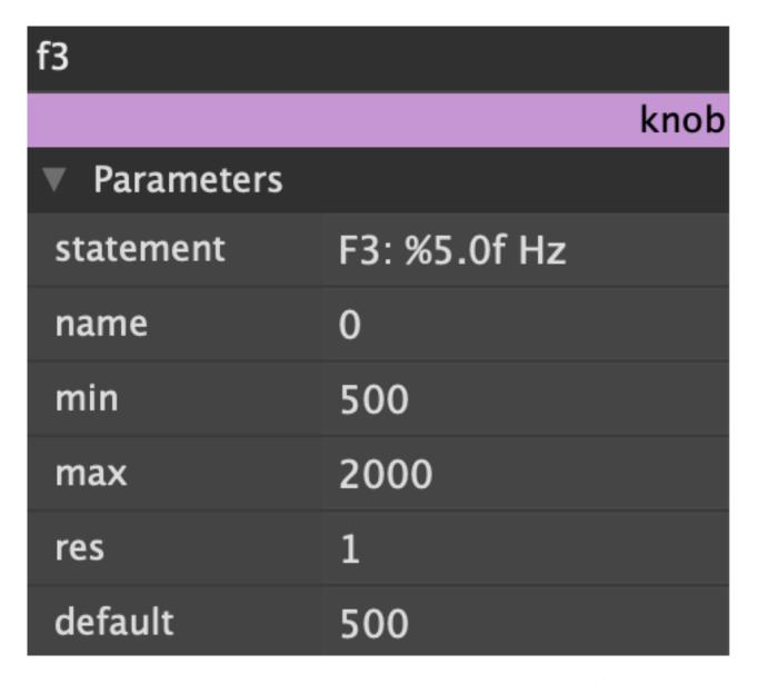
Fig. 6.31 Module editor for knob module, which controls the third EQ band's frequency
