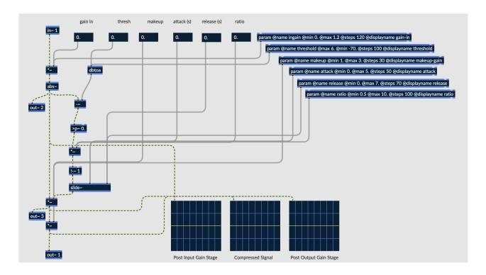
Fig. 6.89 Dynamics compressor with ratio, attack, and release controls
