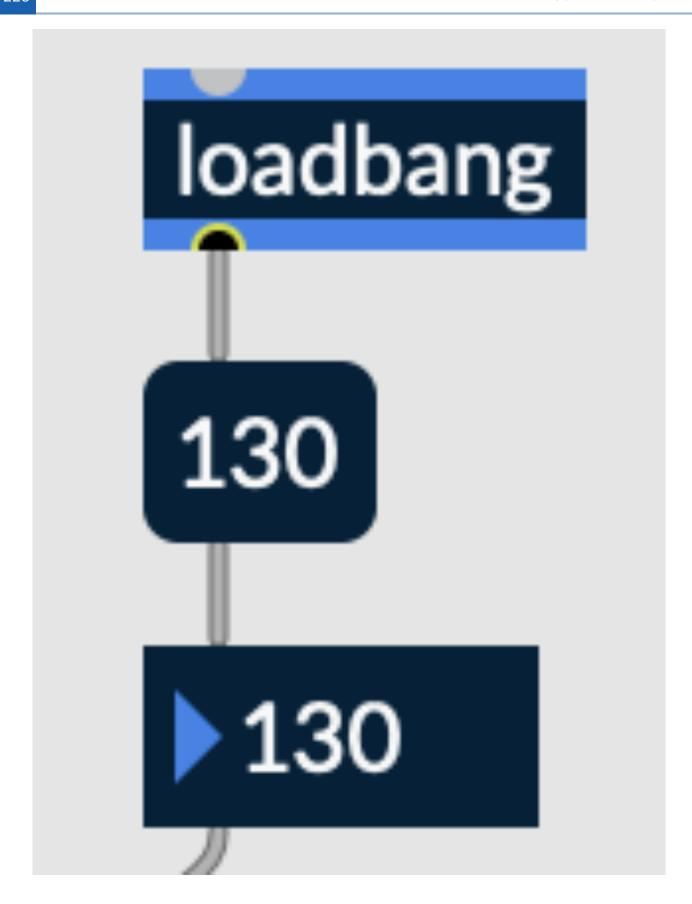
Fig. 6.73 The above objects are used to set the gain to 130 upon loading the patch
