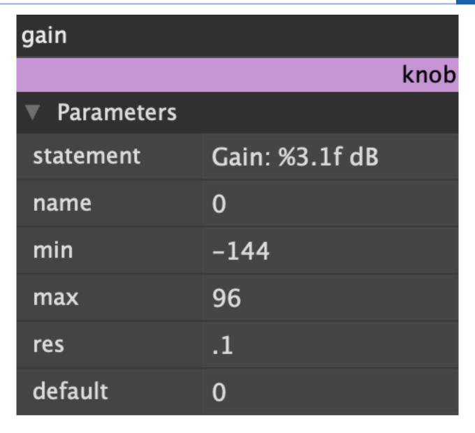
Fig. 6.14 Module editor for knob module, controlling gain
