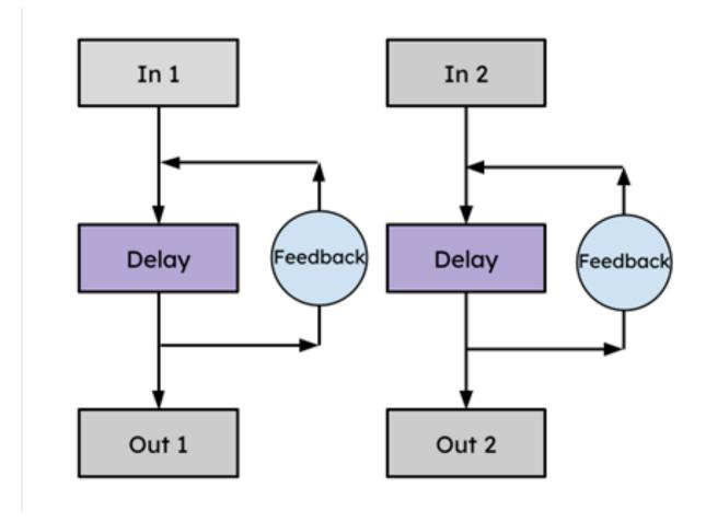
Fig. 6.106 Block diagram demonstrating a stereo delay with feedback
