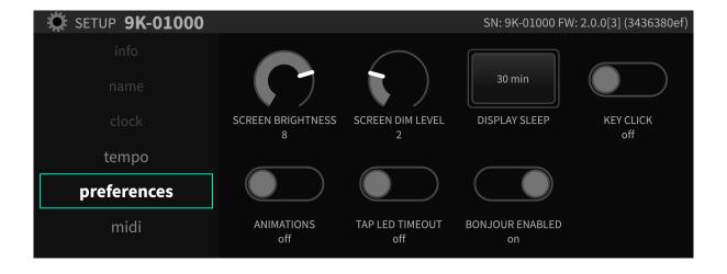
The *Preferences* section controls various aspects of the H9000's display. Use the cursor keys to highlight the setting you wish to adjust, then use the *Enter* key and/or wheel to adjust the setting.
