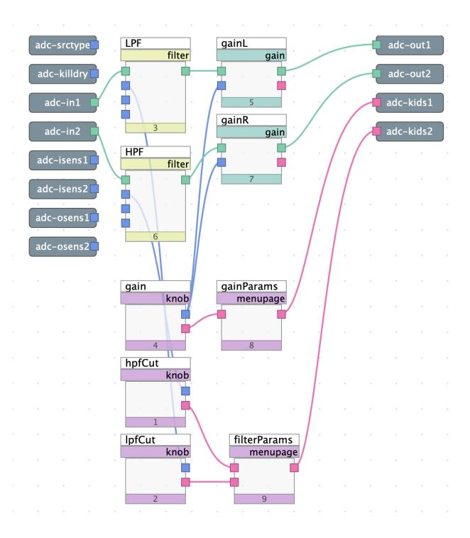
Fig. 6.16 Gain algorithm with filters and interface objects to control cutoff frequency
