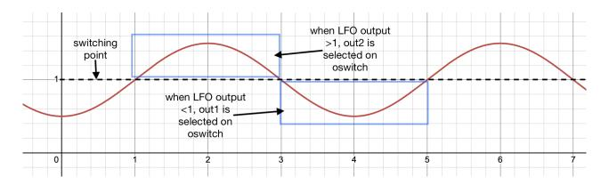
Fig. 6.36 "Vertically shifted" LFO output, using c\_adder module
