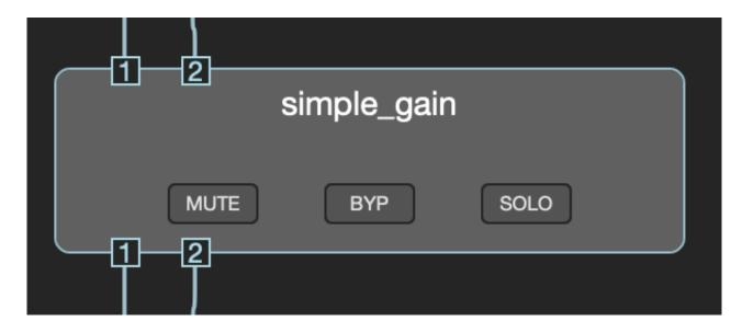
Fig. 6.72 After exporting, the algorithm can be added to the Emote FX chain with the same amount of inputs and outputs as in RNBO
