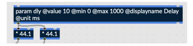
Fig. 6.97 Delay param object, scaled by 44.1 on output
