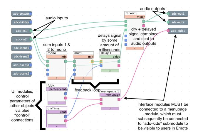
Fig. 6.9 Simple delay algorithm
