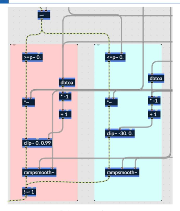
Fig. 6.93 Compression (left) and expansion (right) algorithms, running side by side
