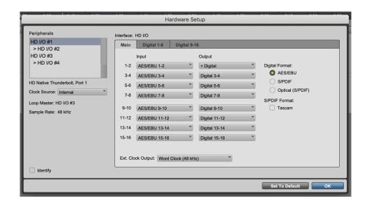
On the left side of the *Hardware Setup* page, your HD devices will appear in the *Peripherals* window. In this case, we have our HD audio interface plugged into the Primary port, and the H9000 plugged in to the Secondary port of the HD Native. In the *Peripherals* window, the HD audio interface will show up as HD I/O #1 and #2, and the H9000 will show up as HD I/O #3 and #4.
