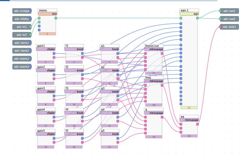
Fig. 6.32 5-band parametric equalizer algorithm, using EQn instead of five EQs
