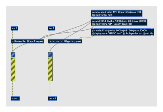
Fig. 6.79 Simple gain, with low and high pass filters applied to the left and right channels respectively
