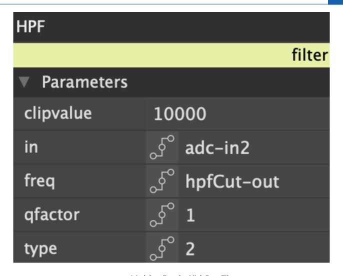
Fig. 6.18 Module editor for High Pass Filter
