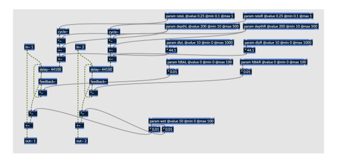
Fig. 6.100 Stereo flanger patch in RNBO
