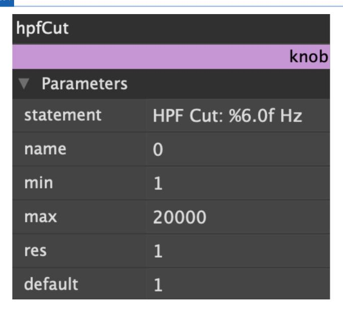
Fig. 6.21 Knob module controlling High Pass Filter cutoff frequency
