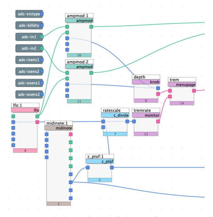
Fig. 6.46 Isolated section of the VSIG algorithm showing tremolo structure
