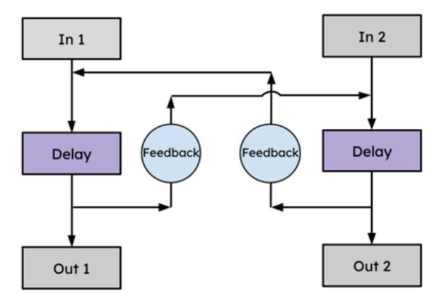
Fig. 6.107 Block diagram demonstrating a stereo delay with crossfeed
