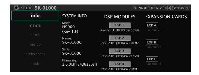
The *Info* screen is a display only; none of its settings can be adjusted. It provides a high-level overview of your H9000 unit, with the following information:
