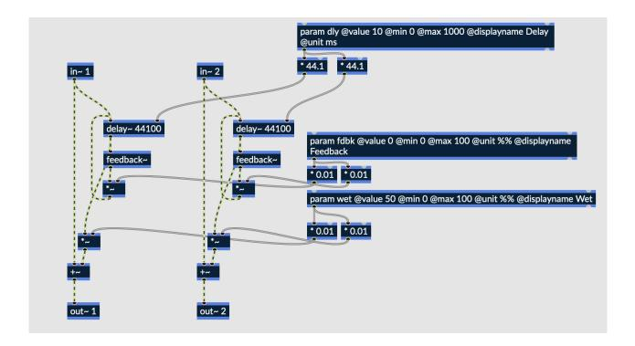
Fig. 6.95 Stereo delay patch in RNBO
