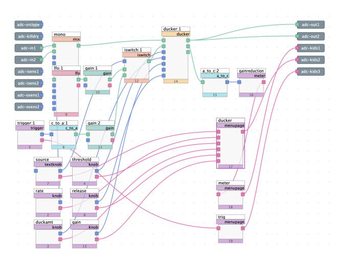
Fig. 6.38 Automatic/manual ducker algorithm
