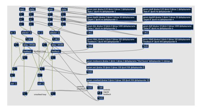
Fig. 6.111 Crossfed stereo flanger with multiple modulation sources
