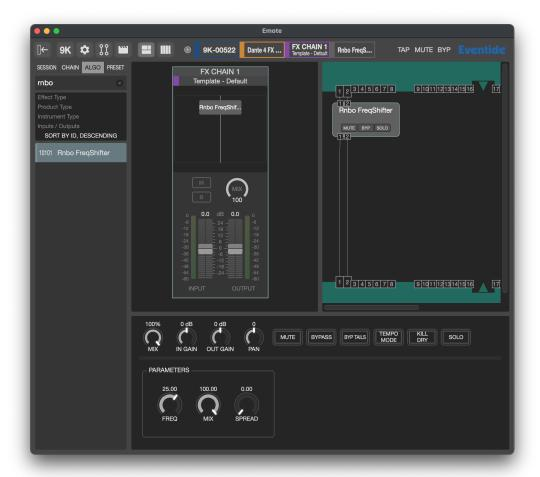
Fig. 6.53 The RNBO freqshifter patch has been exported to the H9000 to algorithm ID slot 10101.
