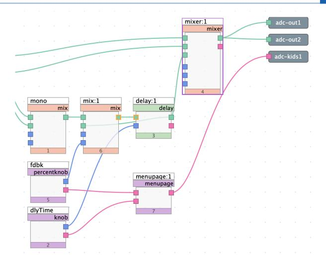
Fig. 6.7 Percentknob and knob module both connected to menupage module via user connections
