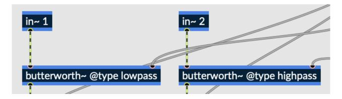
Fig. 6.80 Inputs 1 and 2 both routed into butterworth objects
