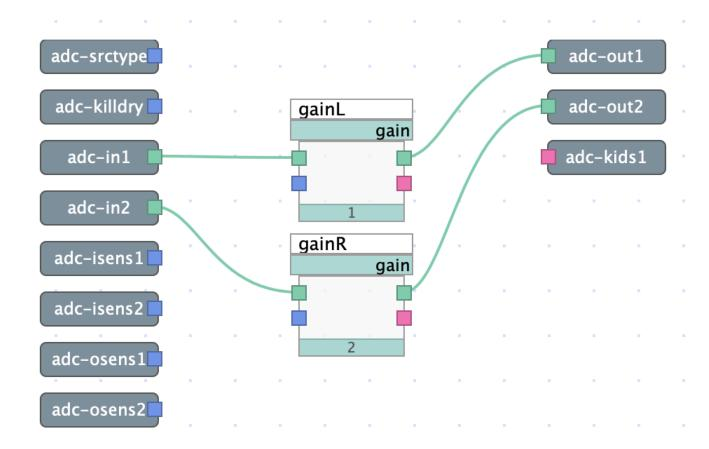
Fig. 6.10 Simple gain algorithm with no user control
