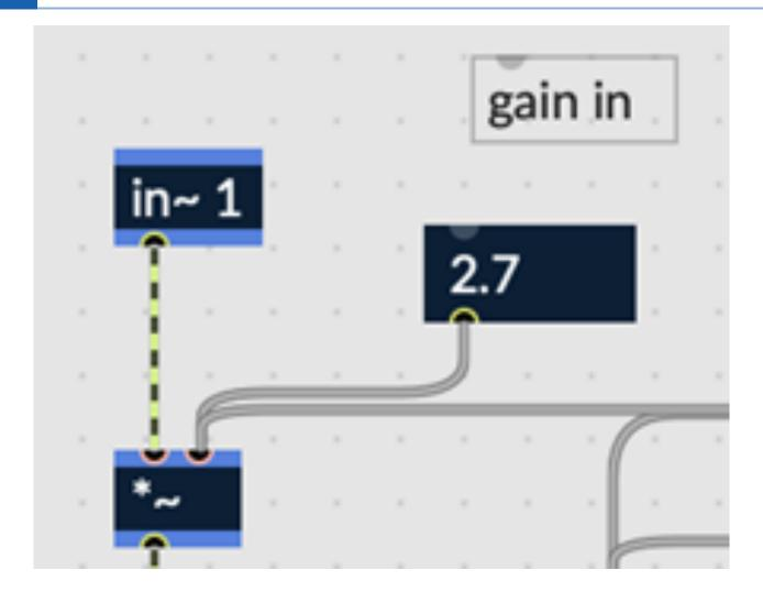
Fig. 6.84 Input stage gain scaling
