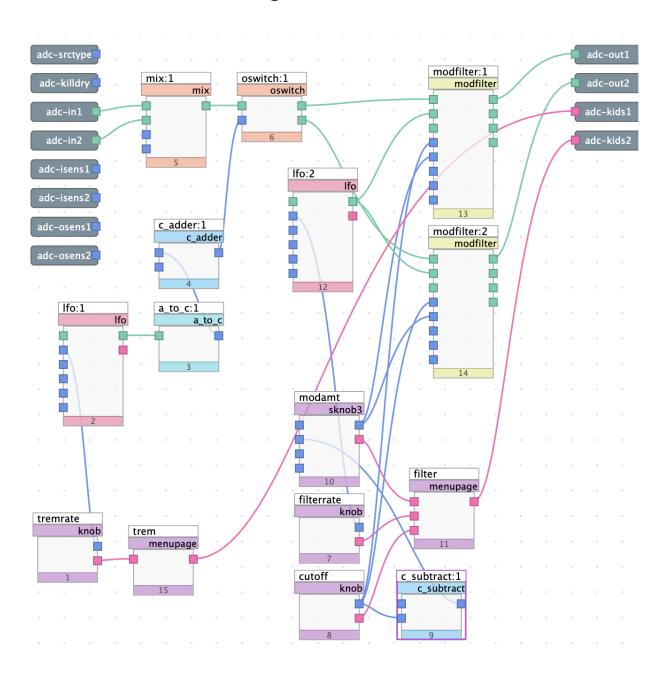
Fig. 6.34 "Stereo Tremolo" esque algorithm using the a\_to\_c module
