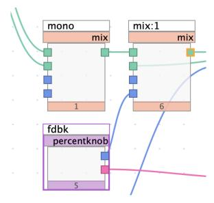
Fig. 6.6 Percentknob module connected to mix module via control connection
