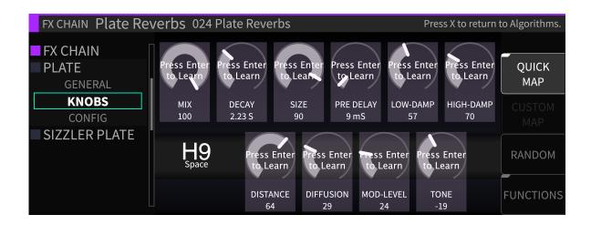
The learn feature is extremely powerful, as it lets you quickly map a wide variety of external controllers to any algorithm parameter. Different aspects of the effects can be adjusted in real time using MIDI controllers, expression pedals, footswitches, control voltages, etc.
