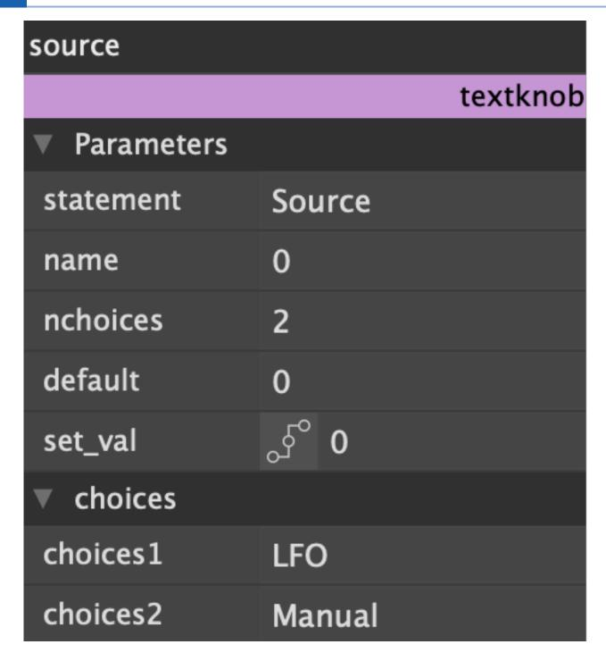
Fig. 6.40 Textknob module editor. Textknobs with only two choices are automatically displayed as a binary switch, as opposed to a drop down menu. Despite both choices being labeled, these labels will not be shown to the user.
