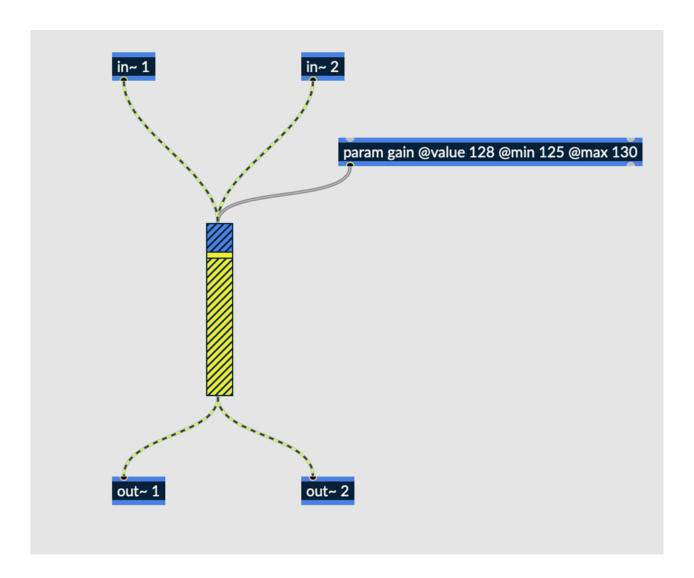
Fig. 6.75 Simple gain patch with UI in Max
