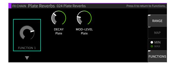
You can use the *Min/Max* soft key to toggle between adjusting the minimum or maximum value of a parameter's range, as indicated by the white and green end cap markers. These Min/Max values only apply to parameters mapped to a Function knob, not the Function knob itself. To set a min/max value for a Function knob, use the *Custom Map* feature in the External Control settings.
