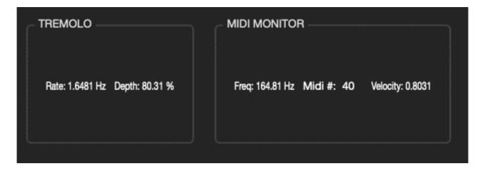
Fig. 6.51 Menus displayed in Emote showing incoming MIDI data and tremolo parameters based off of MIDI data. Notice the relationship between "Velocity" and "Depth," as well as "Frequency" and "Rate."
