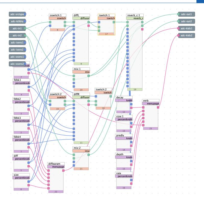
Fig. 6.33 Reverb algorithm utilizing diffusors and the reverb\_c module
