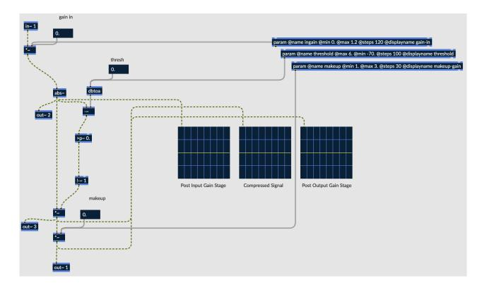
Fig. 6.83 Simple dynamics compressor RNBO patch
